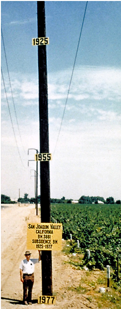
Excessive groundwater pumping often leads to permanent land subsidence. This photo, taken by the U.S. Geological Survey in the San Joaquin Valley southwest of Mendota, California, shows dramatically how much land can compact when aquifers are overdrawn. The signs on the pole mark the sinking of the Earth's surface from where it once was in 1925, 1955, and 1977. The man depicted in the photo is Dr. Joseph F. Poland, a researcher who in the 1970s studied how aquifer overdraft contributed to land subsidence in the West.
